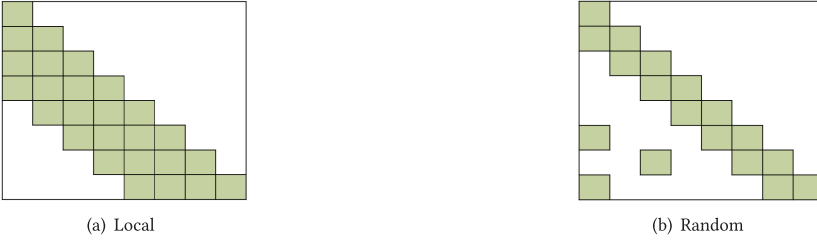
Fig. 3. Examples of temporal mask in temporal aggregation. “Local” means considering continuous snapshots before the current timestep. “Random” means randomly picking historical snapshots before the current timestep. The value is 1 in green boxes and 0 otherwise.
